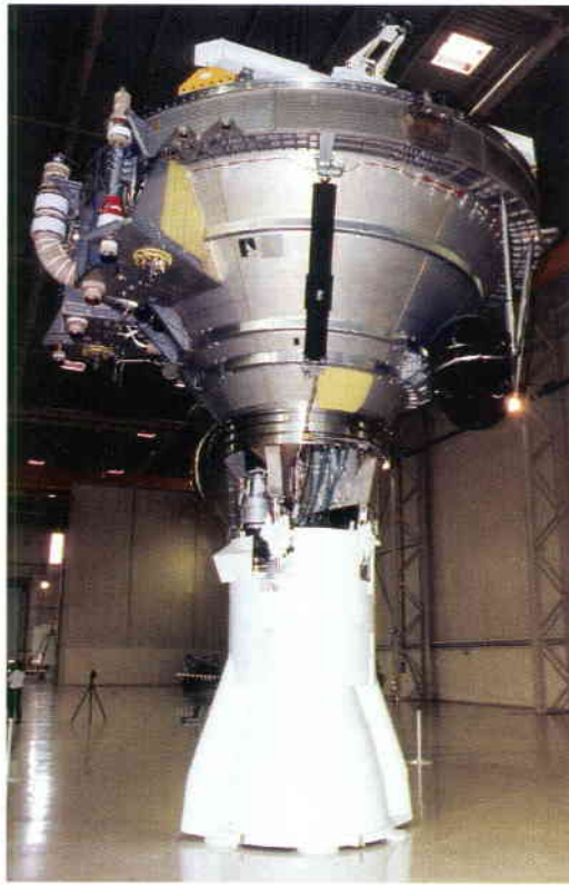
Vibration unit of the aft part of the H155 stage, which has been undergoing testing since October 1992. In white, the Vulcain engine mockup (Photo courtesy of Aérospatiale)
