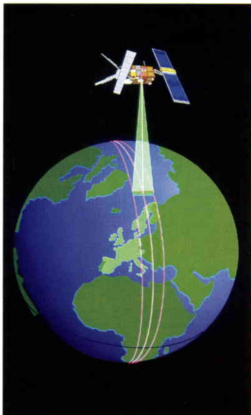
Figure 3. Artist's impression of the GOME instrument's scanning geometry
